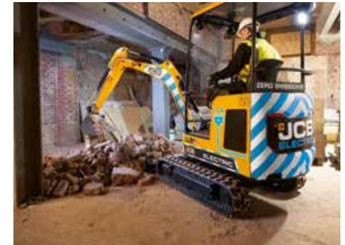
**4** Auto idle makes working efficiently simple by reducing the revs when idle for a set amount of time and therefore utilises the battery in the most effective way.
