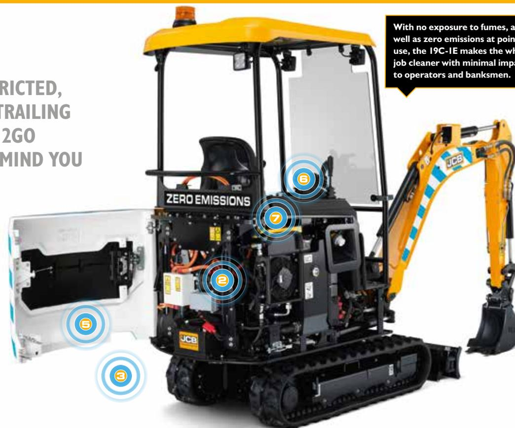
With no exposure to fumes, as well as zero emissions at point of use, the I9C-IE makes the whole job cleaner with minimal impact to operators and banksmen.
